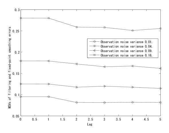
Fig.2 MSVs of the filtering errors  $z(k)-\hat{z}(k,k)$  and the fixed-point smoothing errors  $z(k)-\hat{z}(k,k+Lag)$  vs. Lag,  $0 \le Lag \le 5$ , for the white Gaussian observation noises  $N(0,0.1^2)$ ,  $N(0,0.2^2)$ ,  $N(0,0.3^2)$  and  $N(0,0.4^2)$ .
