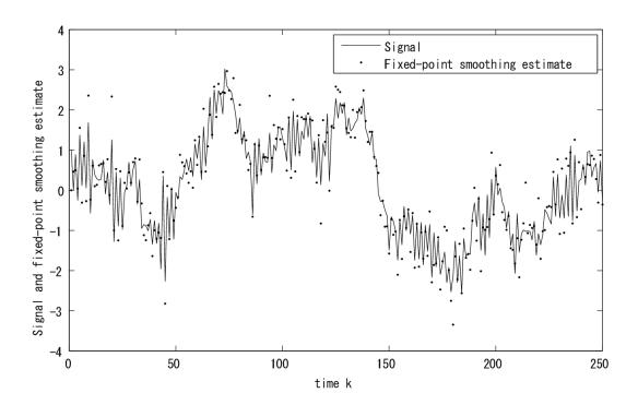
Fig.1 Fixed-point smoothing estimate  $\hat{z}(k,k+5)$  vs. k for the white Gaussian observation noise  $N(0,0.3^2)$  .
